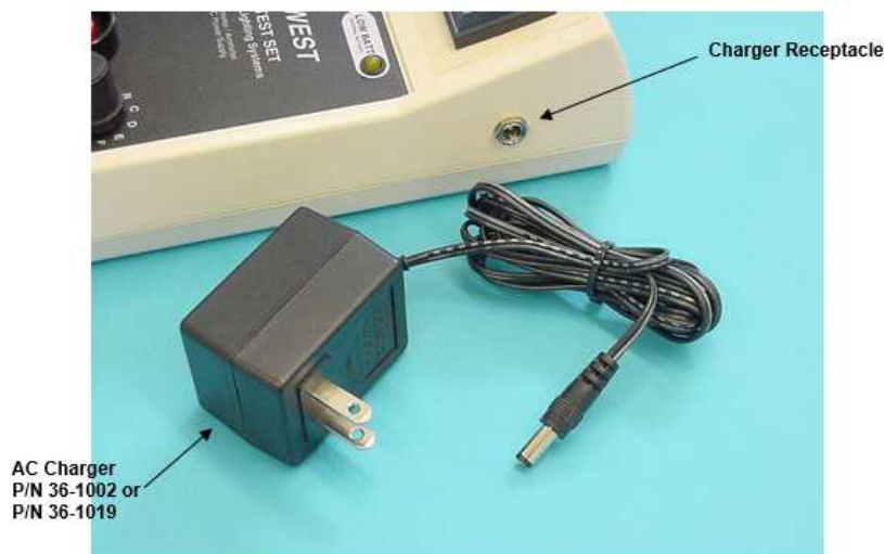
Figure 3. Internal Battery Charging Arrangement
