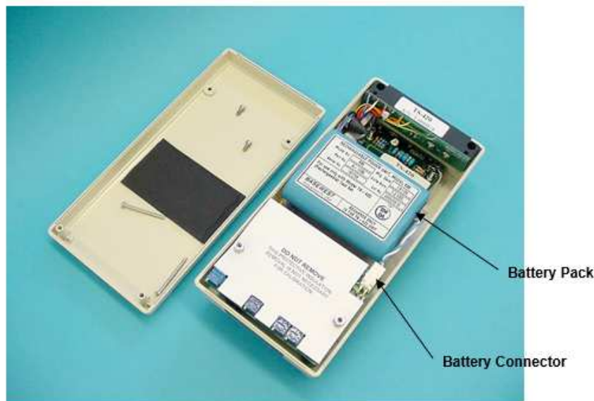
Figure 4. Internal Battery Access
