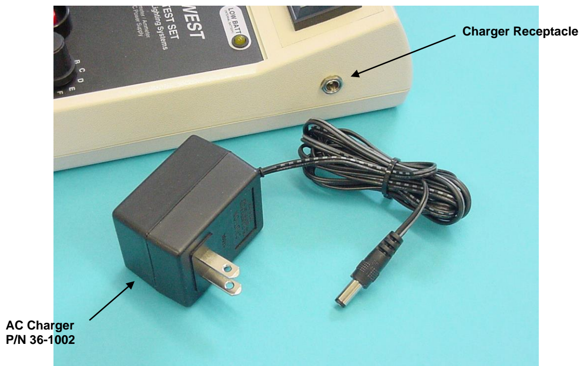
Figure 4. Internal Battery Charging Arrangement
