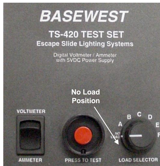
Figure 7. No Load position
