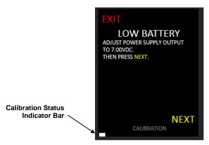
Figure 7. Set Low Battery Level
