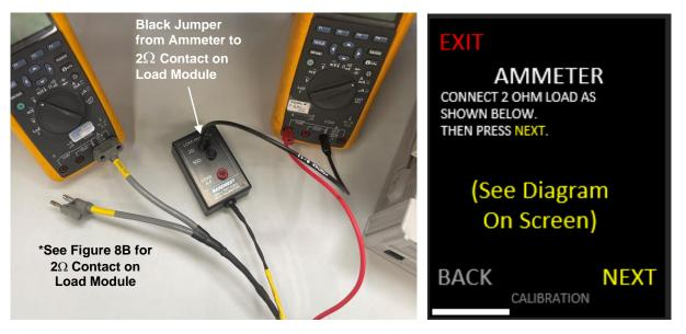
Figure 13. Ammeter (2 $\Omega$ ) Load Module
