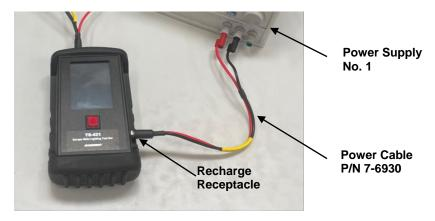
Figure 3. P/N 7-6930 Power Cable Connection
