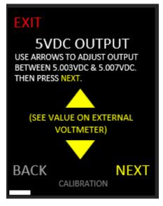
Figure 10. 5VDC Output Adjustment
