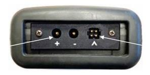
**4-Contact Connector** for battery testing or slide light system testing through battery
