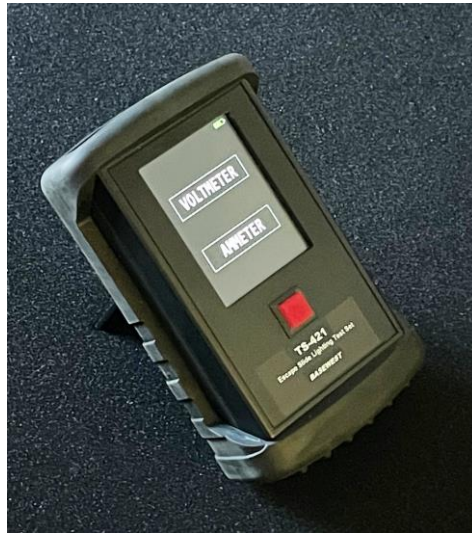
TS-421 Test Set Shown at the Home Screen
