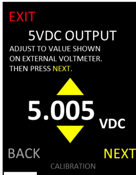
Figure 11. 5VDC Output
