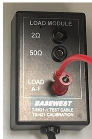
Figure 16B. Load Module Contact - Load A-F
