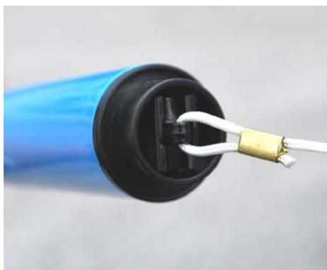
Figure 3 - Installation of Activation Switch Plug
